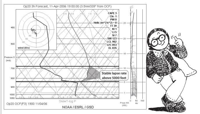
In this three-hour Rapid Update Cycle (RUC) forecast for Ocala, Fla., (KOCF), all three elements of thermal turbulence are present.
