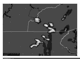
Anomalous propagation (AP) can sneak through the WxWorx filters showing what appears to be intense convective cells (**left**). The Atlanta NWS radar (**lower left**) was the source of the AP in western North Carolina (just north of Toccoa), but a quick check of the Knoxville NWS radar (**lower right**) showed no returns. The precipitation was bogus.
