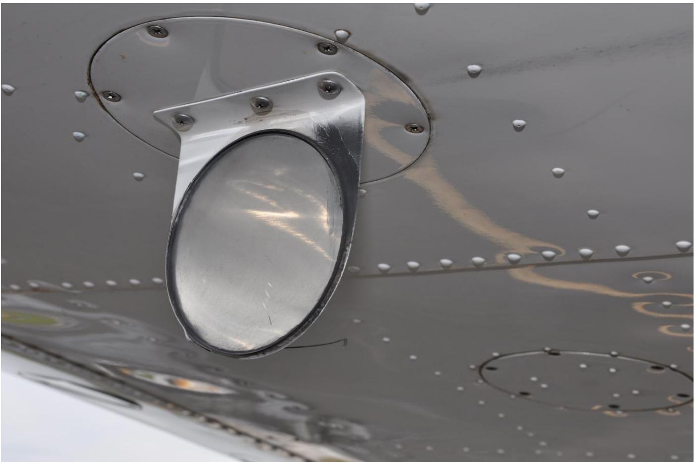
Fig. 18-3: This aircraft-induced lightning strike occurred in a region where there were no convective SIGMETs anywhere close by. The lightning strike entered or exited a mirror that is positioned under this Cessna's wing. This resulted in a bit of black charring on the right side of the mirror. Photo courtesy of Kenneth McLauchlan.
