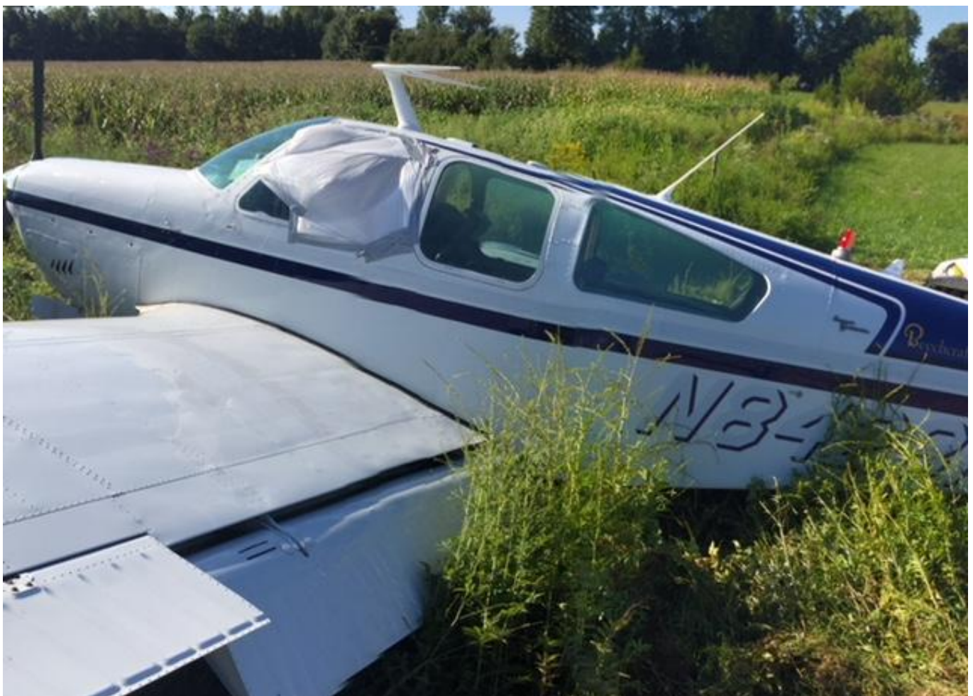
Fig. 18-11: This Beechcraft Bonanza ended up flying into a building low-topped convective cell at 7,000 feet that contained no lightning. The pilot recovered the aircraft at 1200 feet AGL. Notice the shattered pilot-side window. This could have been caused by a loose object inside the cockpit.
