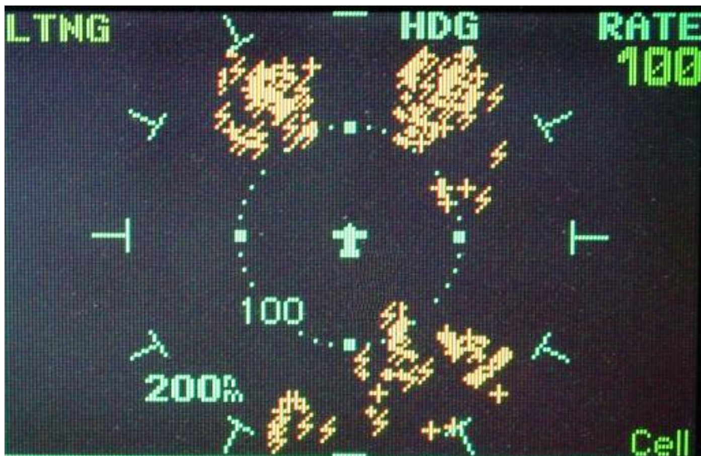
Fig. 18-10: In cell mode the Stormscope attempts to cluster strikes around the location of the cell as shown here on a Garmin 530 GPS.
